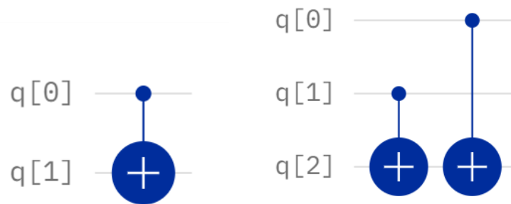
Figure 33: Two possible ways of implementing a quantum XOR-gate. (left) Stores the result of the XOR directly in Qubit1. (right) Stores the result in Qubit2 and requires Qubit2 to be initialized in the |0\rangle state.
