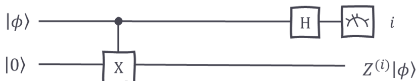
Figure 62: Simplified teleportation circuit. While very similar to “regular” teleportation, the approach is not terribly useful if we consider quantum communication setting, since it requires a control-gate that acts on the input and output qubits, i.e. they have to be at the same location.
