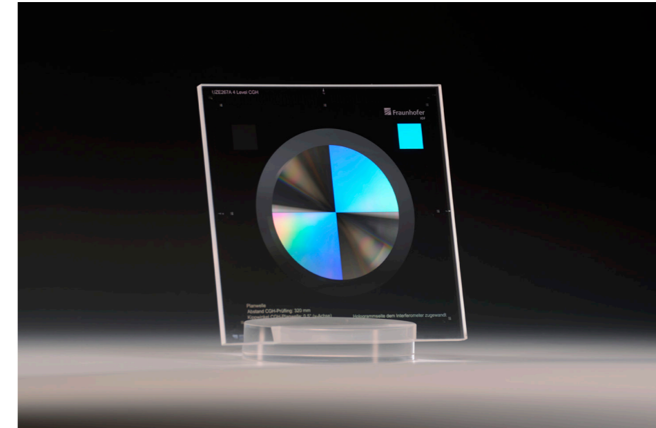
Figure 2: Effective-index asphere test-CGH.
