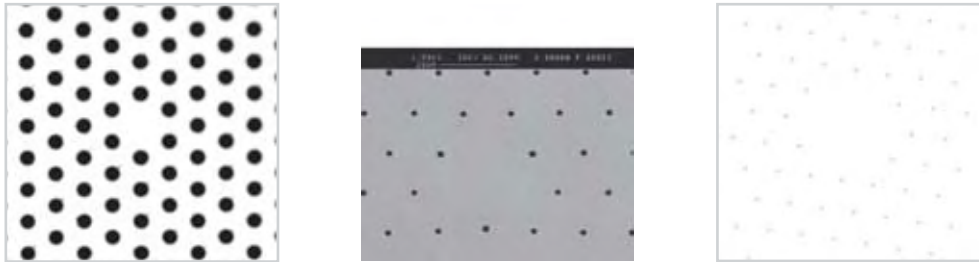
Figure 5: Microscope images of a one, three and seven missing-hole photonic crystal fiber (core region).
