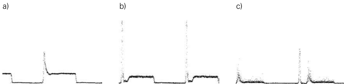
Figure 3 Results of the experiment on the decay of fronts in the case of weak filtering (3 nm), a) 26 km b) 215 km c) 358 km (figures have different scaling).
