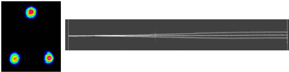
Figure 4 Near-field distribution at the end of a three-dimensional splitter for a wavelength of 800 nm. The exits, which are not in the same plane as the entrance arm, are separated by \sim 40 \mu\text{m} . On the right a polarisation contrast microscope image of the device is shown (stretched in the vertical direction).
