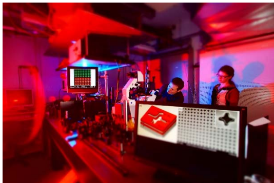
Complexly shaped plasmonic nanoparticles of about 500 nm are examined, using a microscope spectrometer to determine their optical properties which will be exploited for the control of light.
