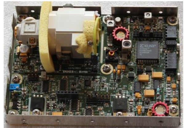
Fig. 3: Open Datum LPRO 10 MHz Rubidium oscillator for time and frequency reference with the so-called Rubidium physics package.
