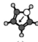
Fig. 1: Sketch of the pyrrole molecule: white (gray, small gray) disks correspond to N (C, H) atoms, respectively, and double bonds are indicated; the permanent dipole moment \mu = 1.93 D of the free molecule is represented by an arrow.
