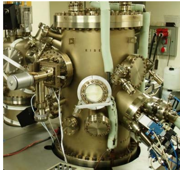
Figure 5: MBE growth chamber equipped with solid-source electron beam evaporators for carbon and silicon, effusion cells and RHEED
