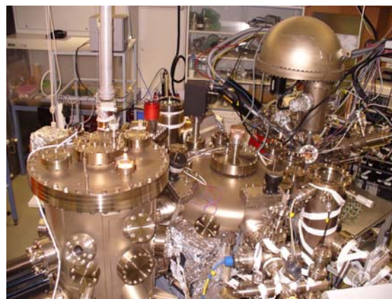
Figure 2: UHV multichamber equipment for surface preparation and characterization by electron spectroscopy and scanning tunnelling microscopy
