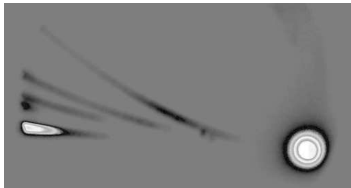
Figure 3.16: Typical parabolic tracks obtained from the MCP. Spectral information can be derived from camera counts vs. horizontal distance to the zero deflection point (bottom right corner).
